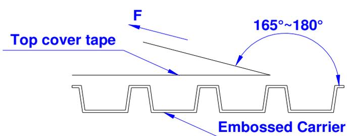
The force for tearing off cover tape is 10 to 130 grams in the arrow direction under the following conditions ( referenced ANSI / EIA - 481 - D - 2008 of 4.11 standard ).
