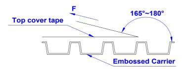
The force for tearing off cover tape is 10 to 130 grams in the arrow direction under the following conditions ( referenced ANSI / EIA - 481 - D - 2008 of 4.11stadnard ).
