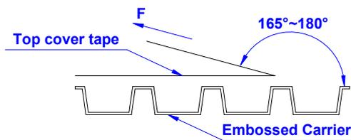
The force for tearing off cover tape is 10 to 130 grams in the arrow direction under the following conditions ( referenced ANSI / EIA - 481 - D - 2008 of 4.11 standard ).
