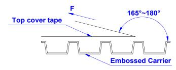
The force for tearing off cover tape is 10 to 130 grams in the arrow direction under the following conditions ( referenced ANSI / EIA - 481 - D - 2008 of 4.11stadnard ).
